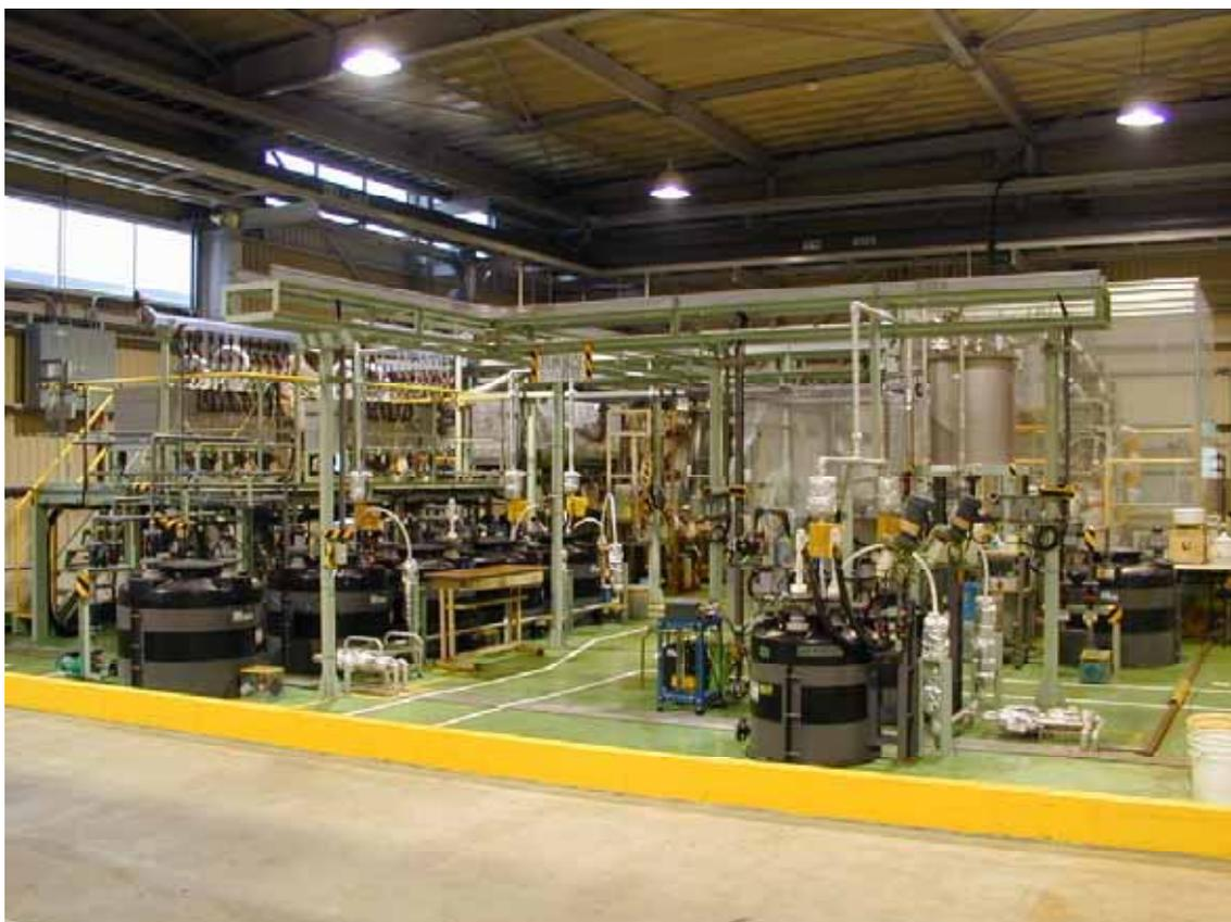
NEW HYRDOMEATTURGICAL COPPER REFINING PROCESS (Sumitomo Metal Mining)
