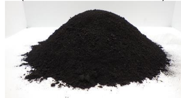
In-process recycled material (used LIB after neutralization)
