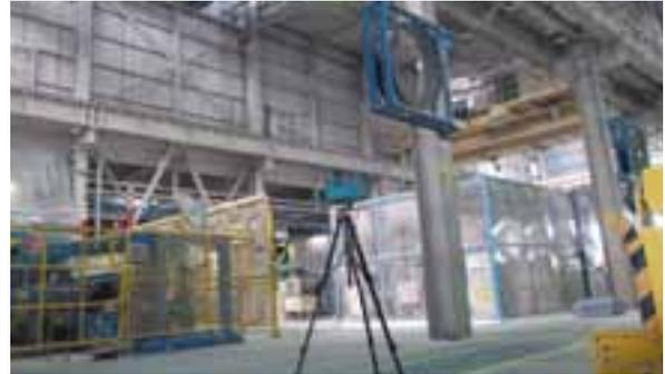
▲ Fans and a dust counter (center) used to measure dust particles. Sources of dust are covered by sheets.
