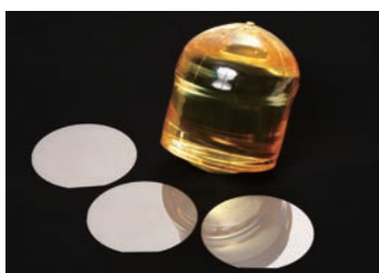
LT substrates (crystal and wafer) LT: lithium tantalate
