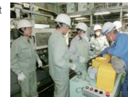
On-site hazard simulation—Chain entanglement hazard simulation
