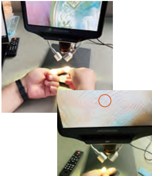
If you rub a coin against your fingertip and examine it under a microscope, you can see fine copper particles attached to your fingertip.
