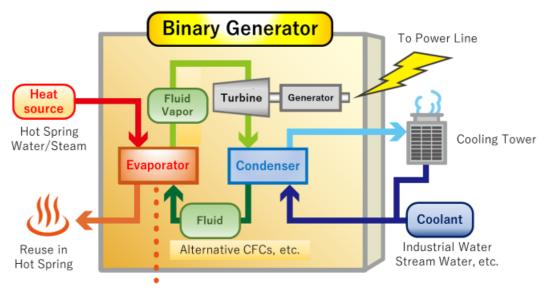
The heat from the hot spring is used to heat and vaporize the fluid, and the vapor pressure rotates a turbine that generates electricity.
