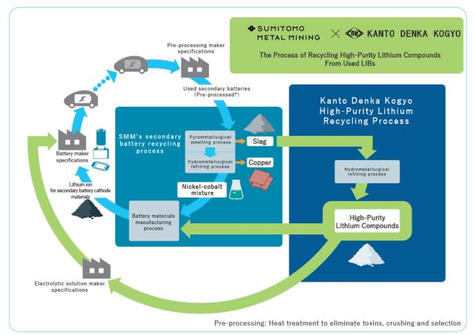
The process we have jointly-developed uses KDK's metallurgy processes to recover high-purity lithium compounds from the slag containing lithium that occurs in our secondary battery recycling process. These high-purity lithium compounds are then reused in LIBs.
