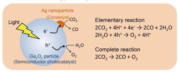
Close-up of an Ag nanoparticle-loaded semiconductor photocatalyst particle
