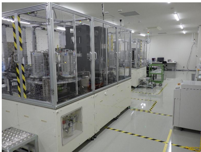
Equipment at GRANOPT's second plant for inspecting the optical properties of Faraday rotators
