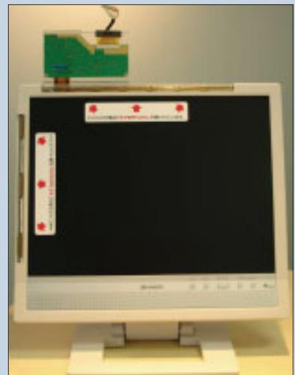
Copper-clad Polyimide Film used in Flat Panel LCD TV
