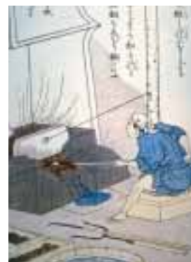
The Nanban-buki smelting technique allowed the separation of both copper and silver from mineral ore.
