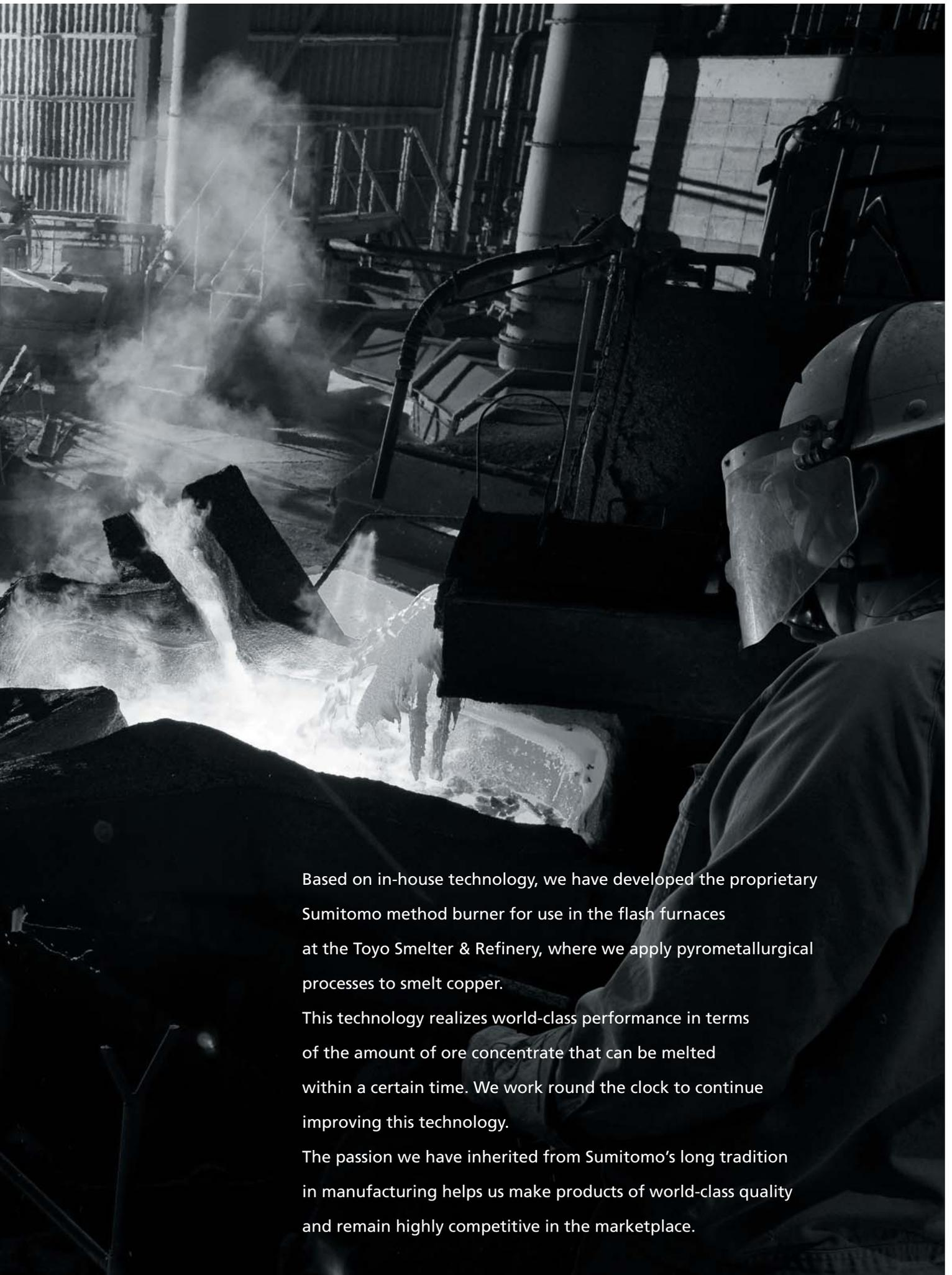
Based on in-house technology, we have developed the proprietary Sumitomo method burner for use in the flash furnaces at the Toyo Smelter & Refinery, where we apply pyrometallurgical processes to smelt copper.
